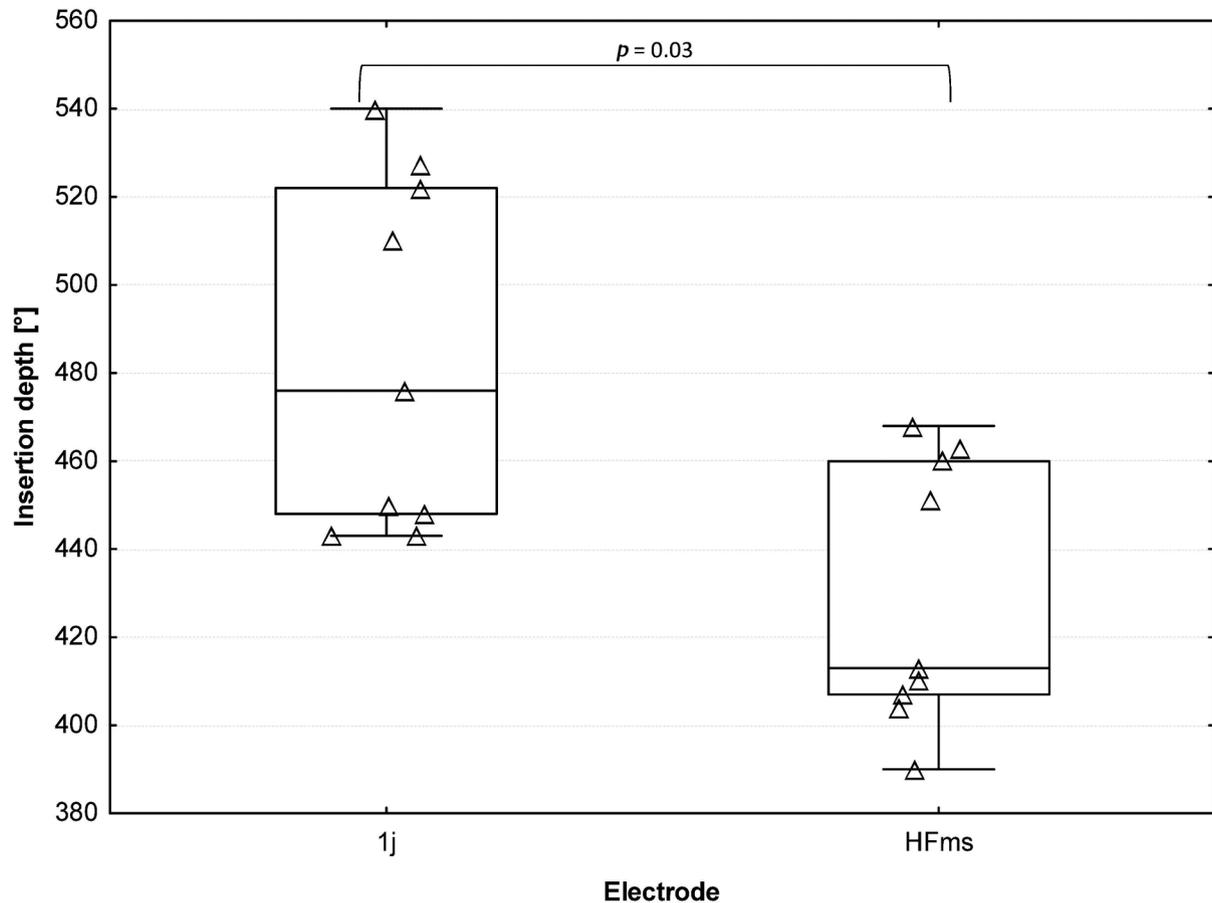
**Fig. 3** Angular insertion depths for each electrode array type.  $N = 9$  ears in both groups. Box plots show the median, first, and third quartiles. Whiskers show the maximum and minimum values.
