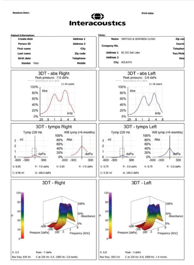
**Fig. 9** Wide band tympanometry test done in the Interacoustics wide band tympanometer in the authors' clinic. The patient is a 13-year-old boy who presented with tubo-tympanic catarrh bilaterally. The test is after a course of steroids. The top graphs are the 2D absorbance graphs, in the middle are the traditional tympanograms at 226 Hz and 1000 Hz, and at the bottom is the 3D composite graph.
