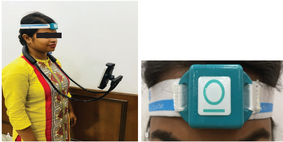
Fig. 2 (A) The V-Gym rehabilitation being carried out using the patient's mobile phone with the requisite rehabilitation app installed in it. The patient can walk around while performing the rehabilitation exercise. (B) The hardware for the V-Gym rehabilitation consists of just the headband with the gyroscope fitted on it.
